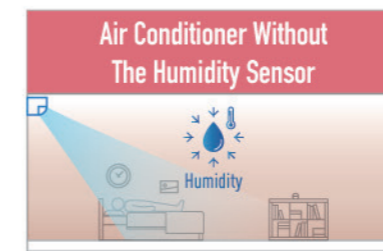
Without the humidity sensor, relative humidity increases in the room during stable operation causing uncomfortable sleeping environments.
